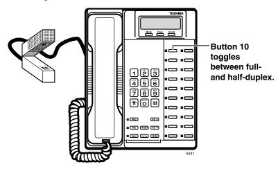
Figure 9 Button 10 on the Full-duplex Speakerphone
